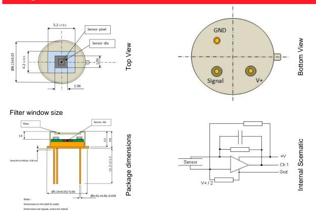
Note: Ensure that the sensor base is not in contact with the PCB in order to avoid shorts.
